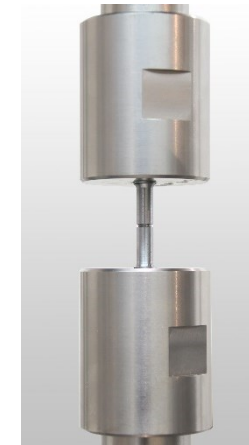
Tensile test acc. ASTM E8 → NFS (notched fracture strength)
