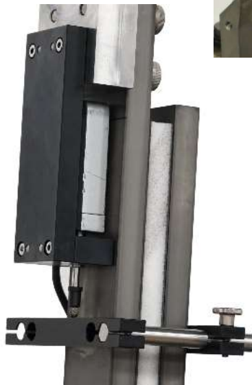
Opto-electronic measurement transducer used for core shear testing
