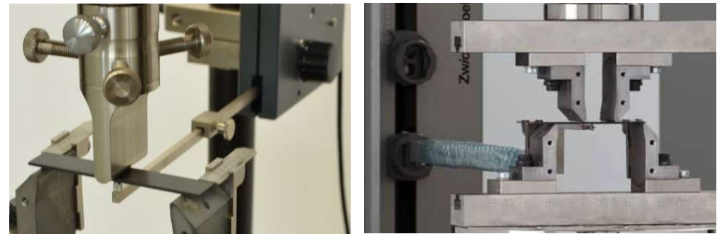
Deflection measurement with deflectometer (left) or with makroXtens and sensor arm for flexure tests...
