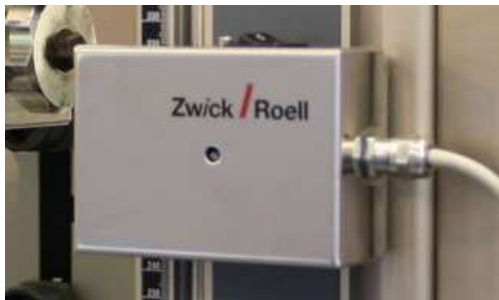
...connected to preconfigured strain gage box...
