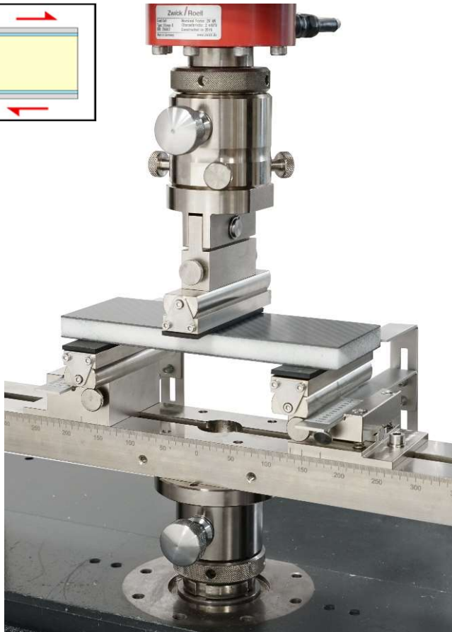
standard 3-point flexure setup as per ASTM C 393
