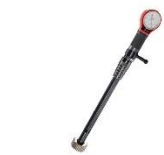
/N6 - Hardness testing in drill holes
