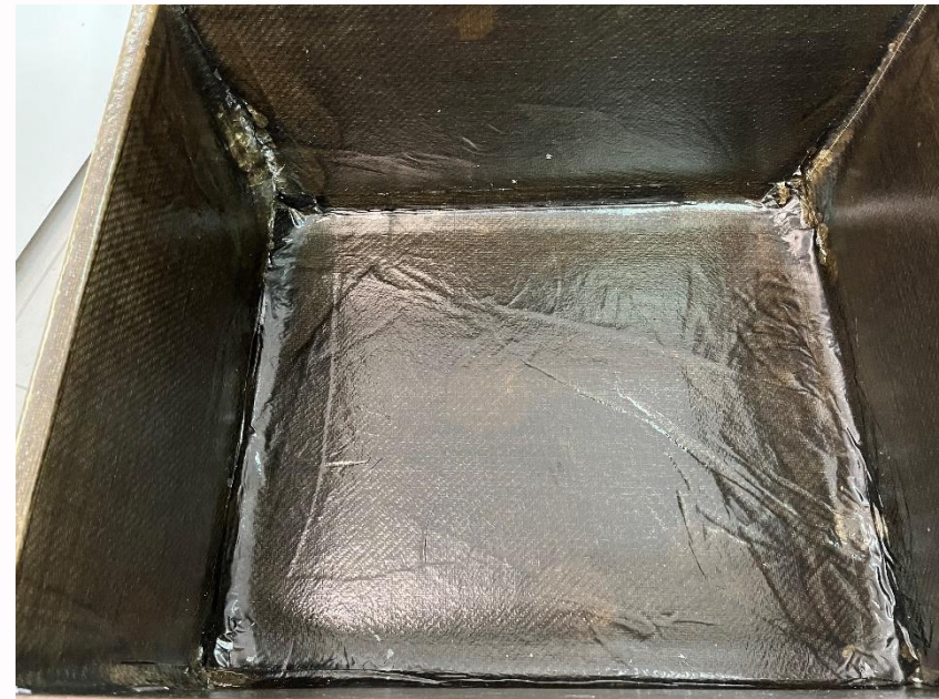
High resin content of Prepreg >50 wt%
