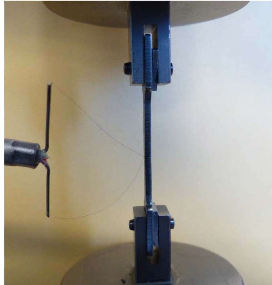
Temperature measurement with thermocouple
