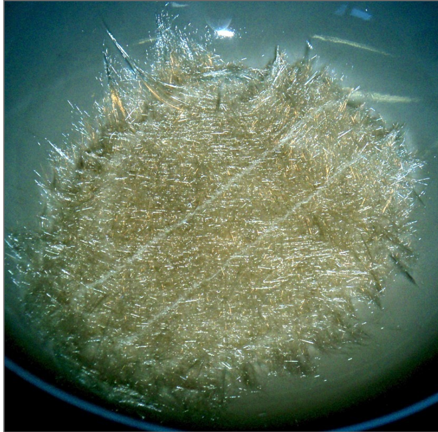
„AOI “ after calcination: undestroyed fibres in the boundary area
