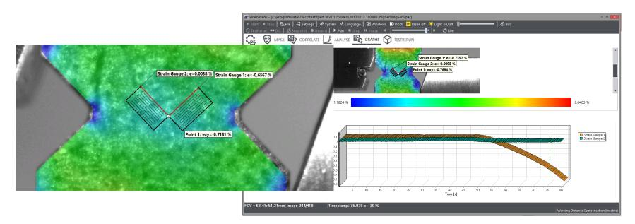
Example: losipescu test (shear test on v-notched composite specimen) with 2 virtual strain gauges.
