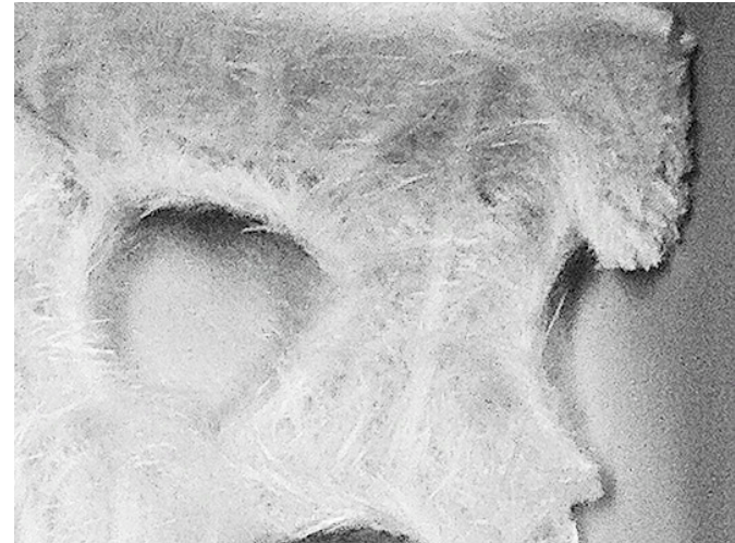
Part of seat bracket for German OEM after calcination
