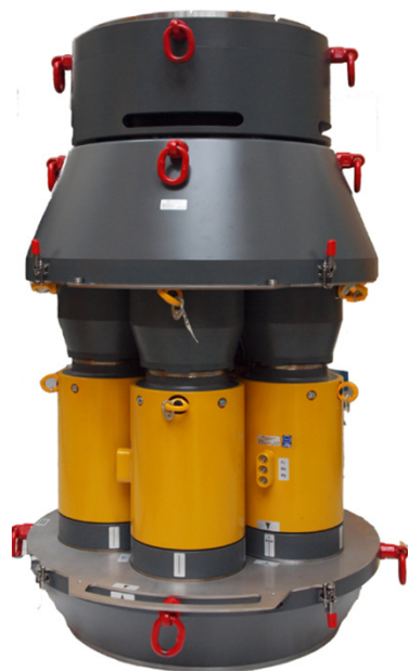
Calibration of the Transfer-Standard in PTB's 16,5 MN FSM
