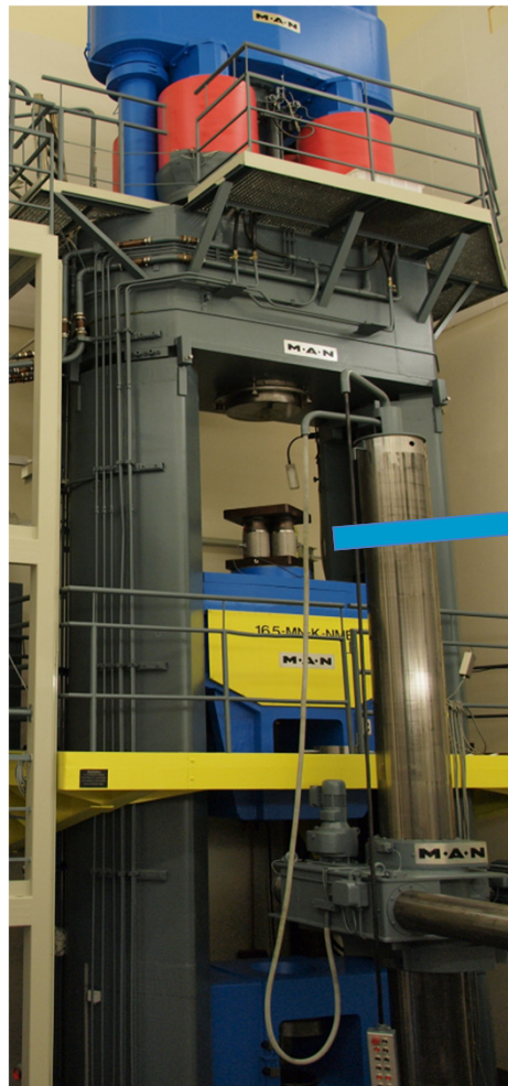
Calibration of the Transfer-Standard in PTB's 16,5 MN FSM
