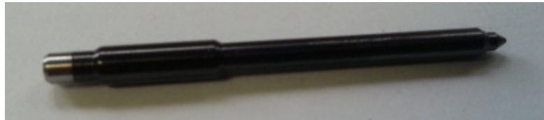
Injection needle for diesel engines (DLC coated)
