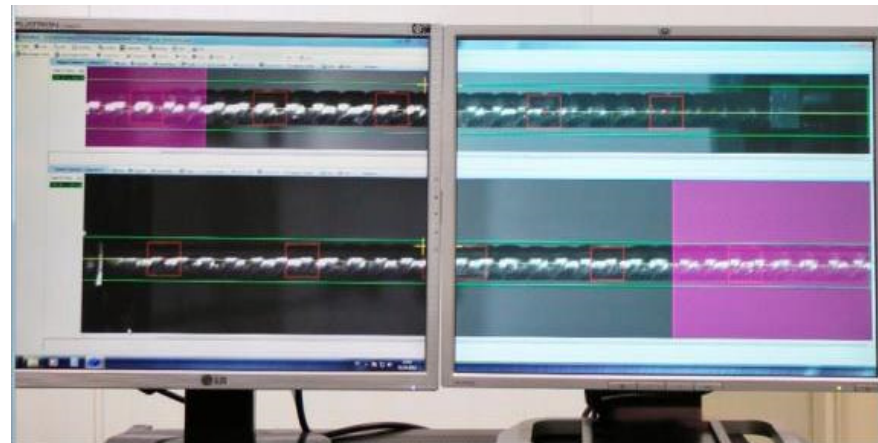
Strain distribution: the red squares mark the gauge marks
