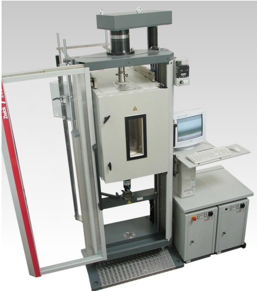
Z050 Allround, torque drive 200 Nm
