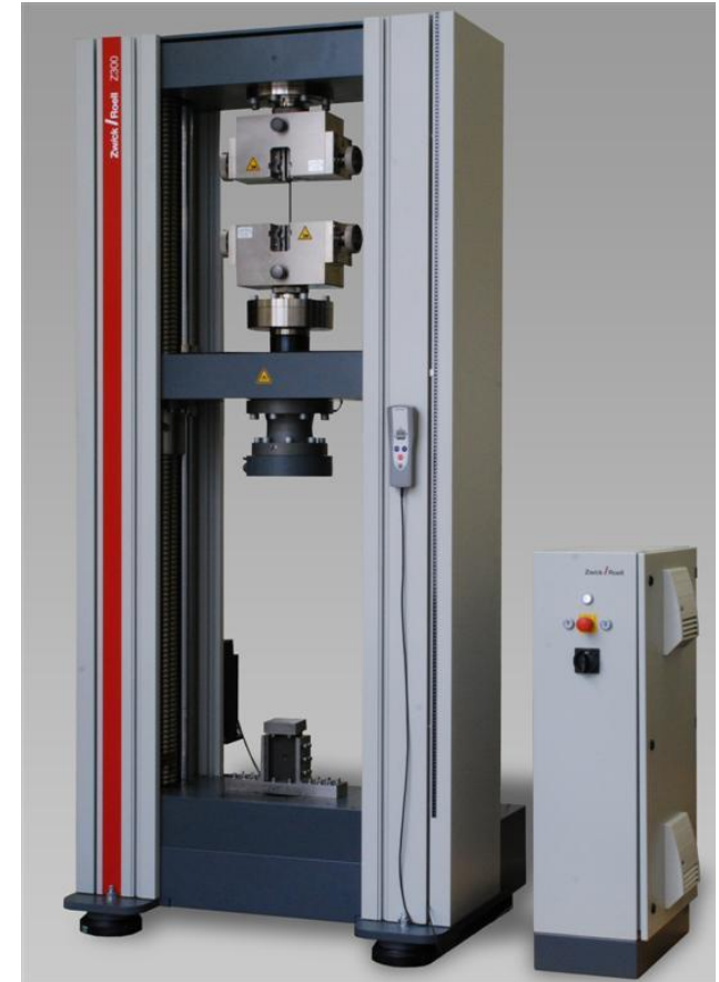
Capacities of up to 2000 kN with electro-mechanical drive system.
