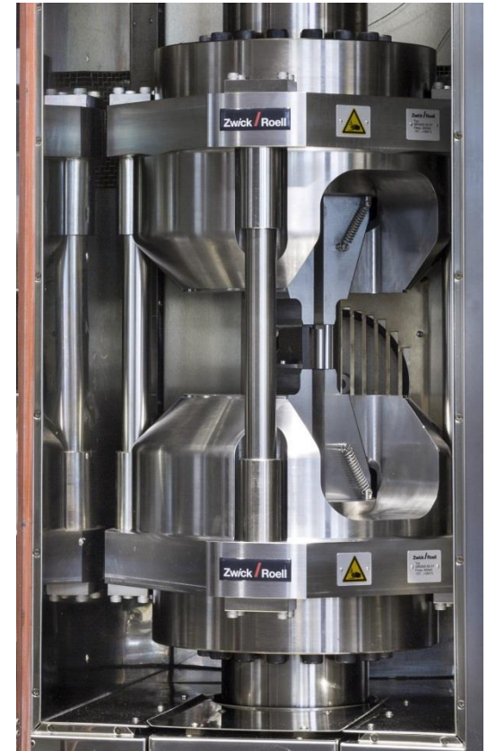
Laterally guided hydraulic gripping system for up to 600 kN
