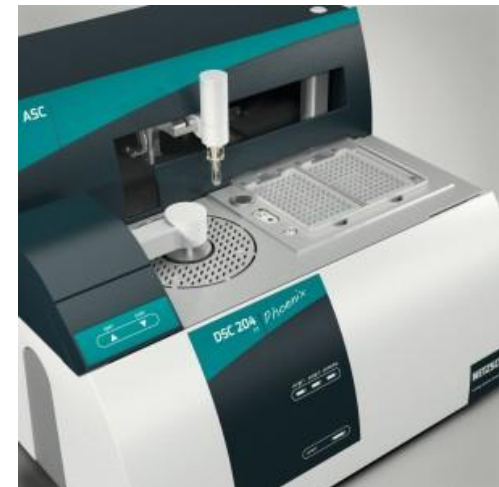
DSC 204 F1 Phoenix with automatic sample changer Temperature range: -180°C....700°C
