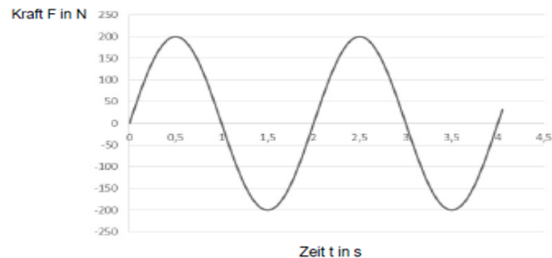
Typical loading cycle for conductor
