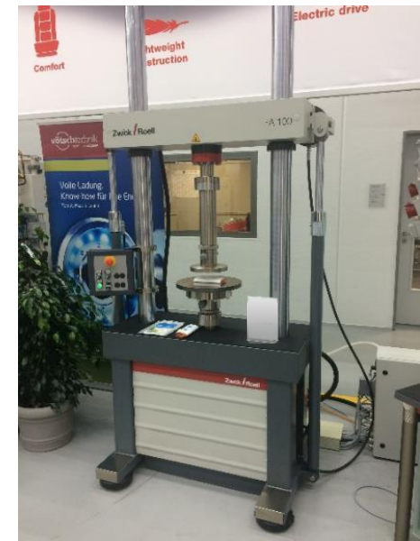
HA 100, 100 kN testing machine prepared for integration of a temperature chamber (HL6)
