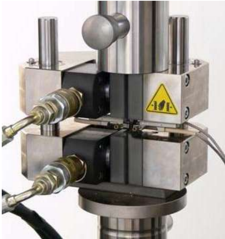
Double sided clip-on extensometer placed on a specific holder
