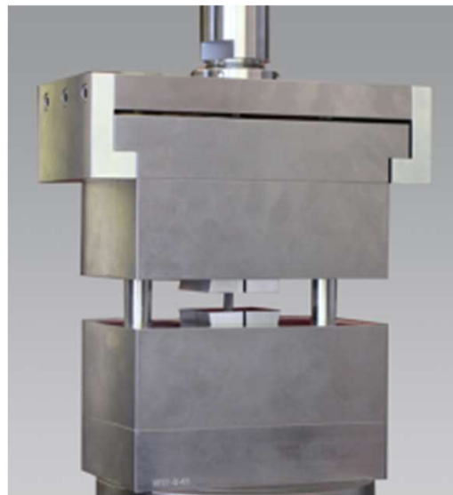
ITRI fixture described in ASTM D 3410
