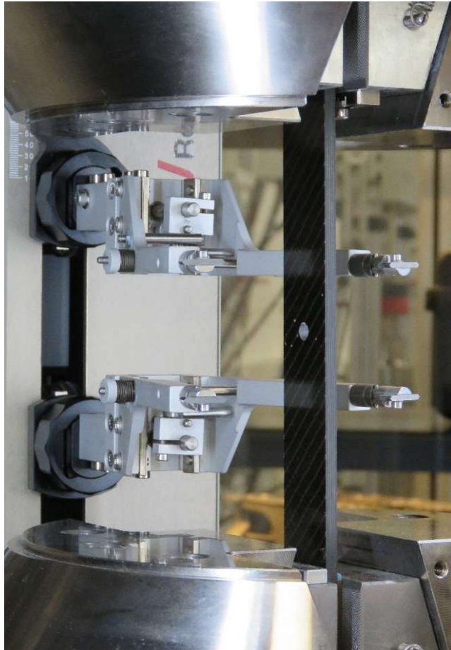
Open-hole tension test
