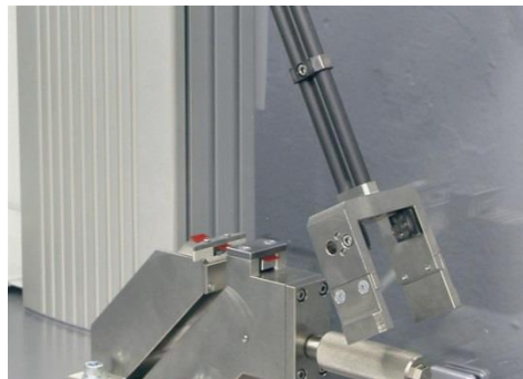
Tensile Impact Here: ISO 8256 method A
