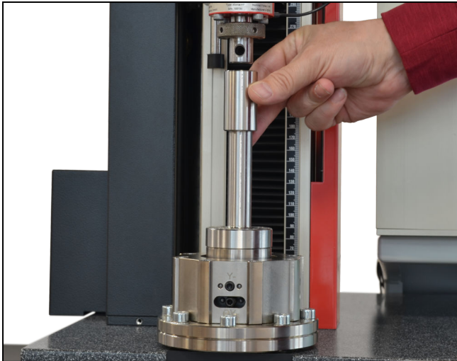
Alignment fixture for axial offset and angle correction with adjustment rod, Fmax 5 kN
