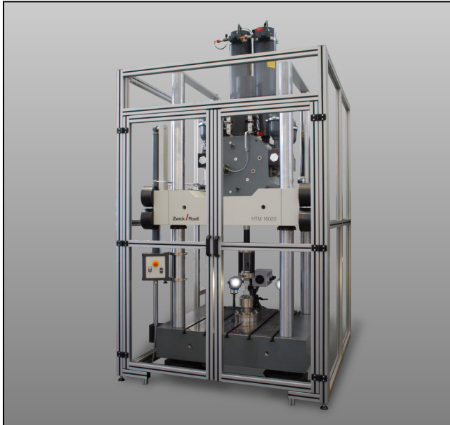
HTM 16020 high-speed testing machine
