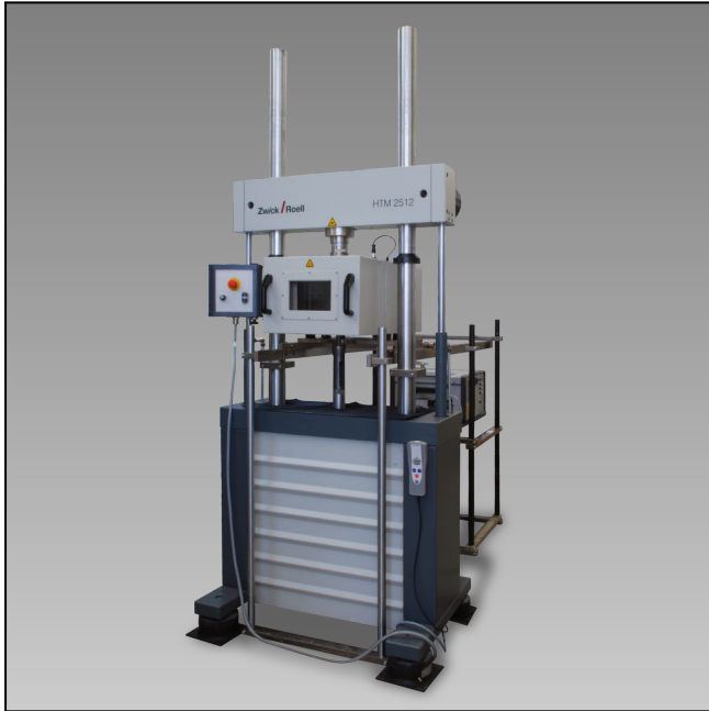
HTM 2512 with temperature chamber
