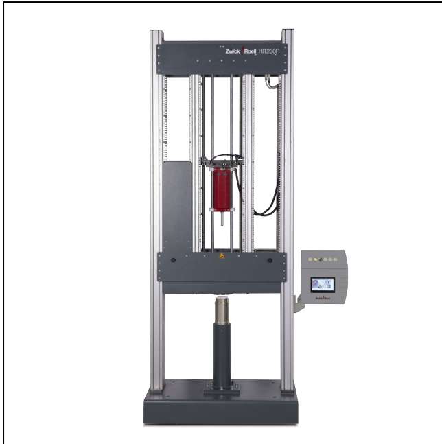
Amsler HIT230F, multiaxial puncture test
